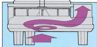
**TITAN's** vortex impeller guarantees reliable, low-maintenance performance. The powerful vortex action created by the recessed impeller draws liquids and solids through the body while back vanes provide seal protection.
